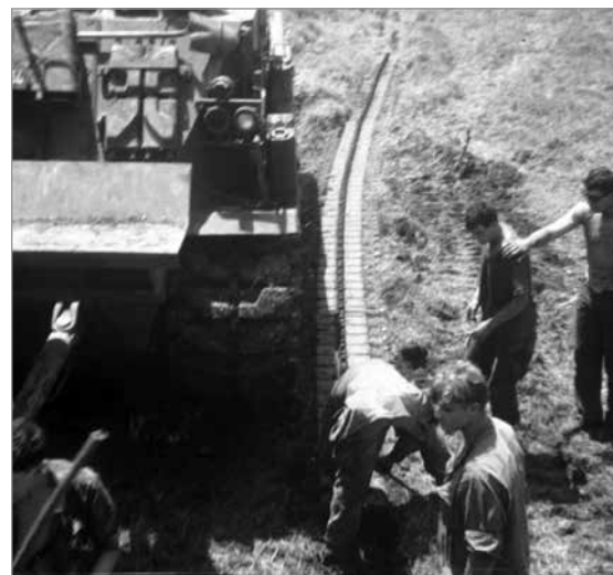
BRAVO Co. Tank Retriever assisting BRAVO 33 with track lost due to a land mine, April 1969.
